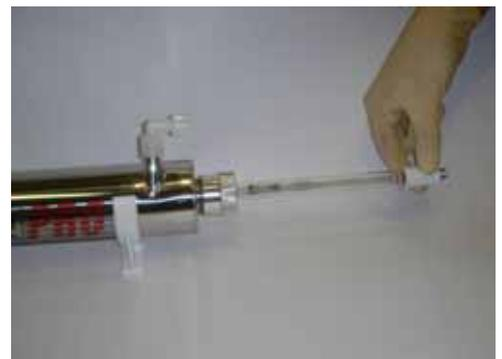
*Connect the female 4-pin plug from the ballast to the pins on the lamp.*
